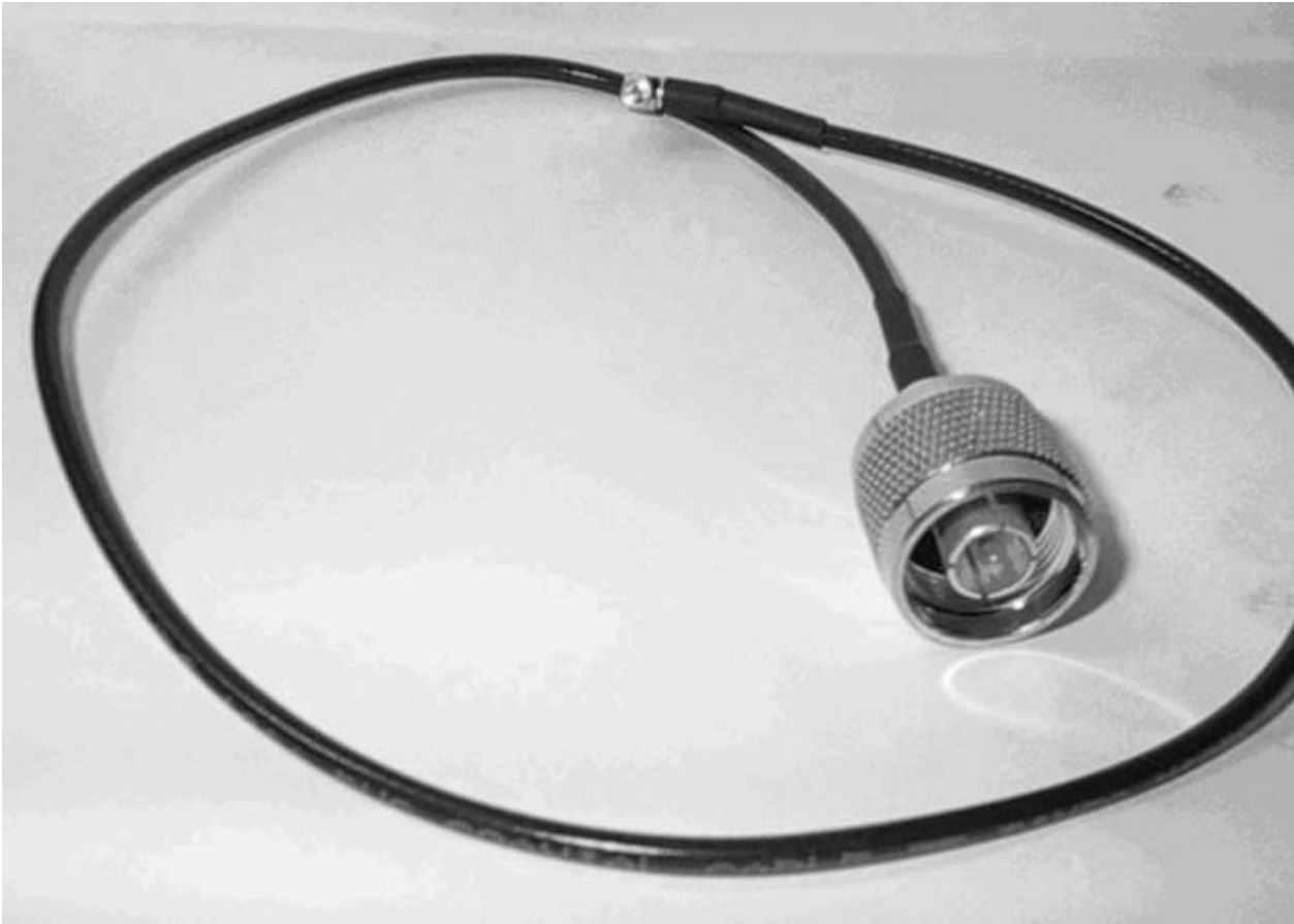
Figure 10.18 A Common 10" Pigtail with "N" Connector and MMCA (PCMCIA) Connector
