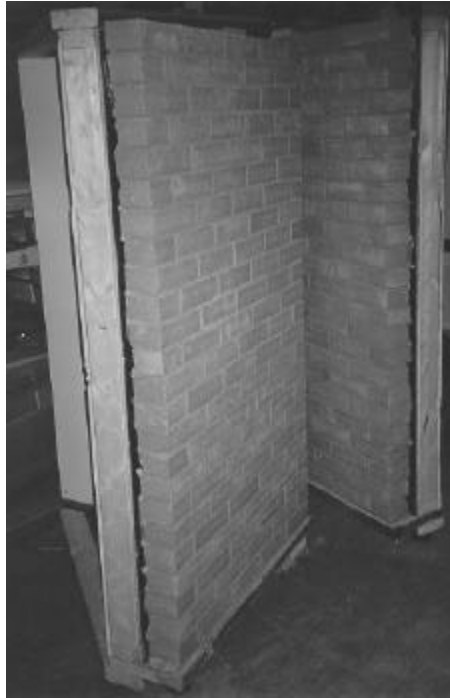
Figure 1 - Concrete Brick with Wood Stud Backup Wall Specimens
