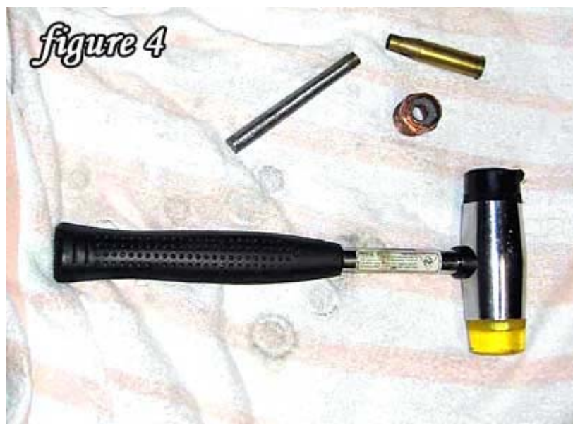
Figure 4. Pretty much all you need for de capping your Berdan brass. A rubber/plastic mallet works better than a metal hammer.
