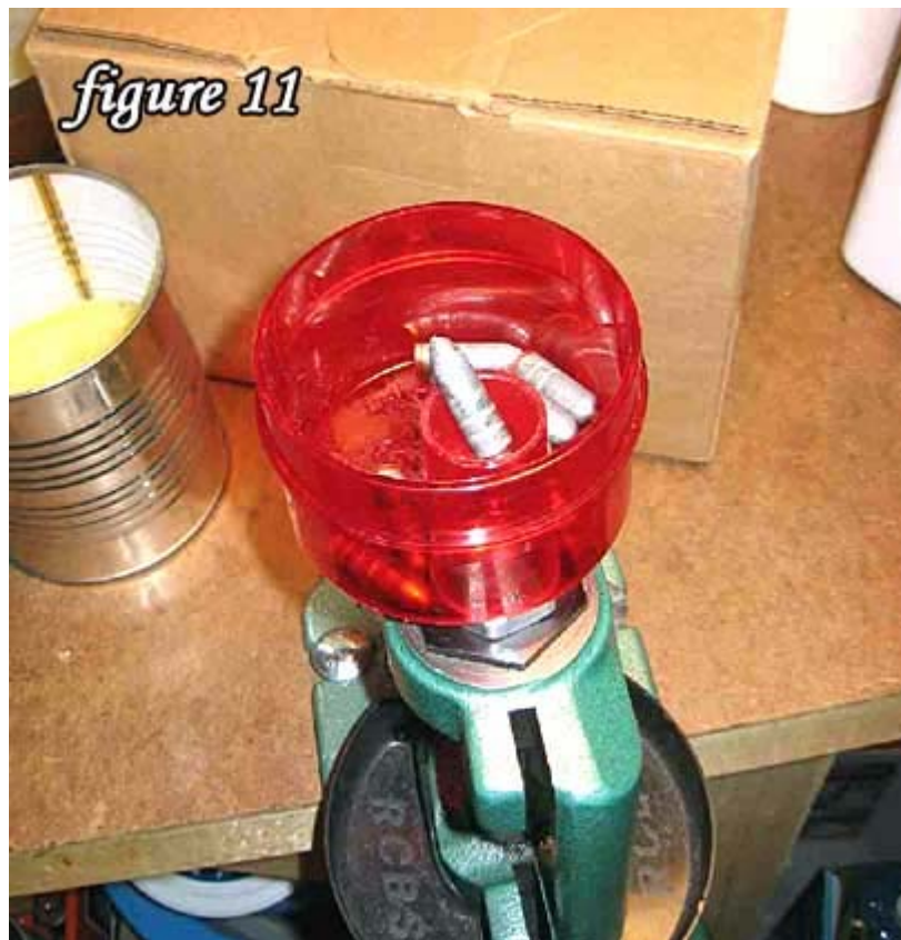
Figure 11. A view down into the holding cup. As the bullets are sized, they are pushed up and out into the cup.
