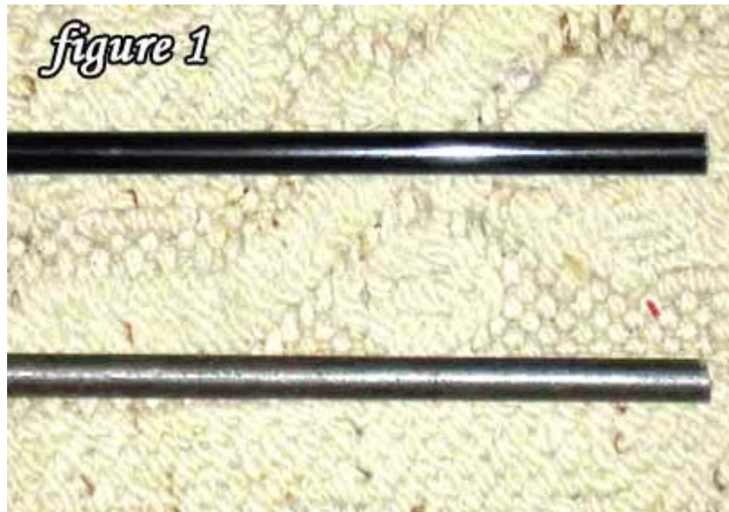
Figure 1. Both rods are 3/8" diameter. The one on the bottom is mild steel. The one on top is solid fiberglass. The fiberglass was easy to file down but did not last long. The mild steel was harder to file down, but lasts pretty much forever.
