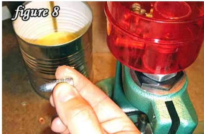
Figure 8. I spread a small amount of lube along the grooves with my fingers prior to sizing the bullet. Do not try to size unlubed bullets. Alternatively, Lee's liquid Alox could be used to lube the bullets, before and after sizing.
