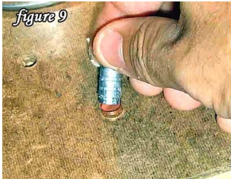
Figure 9. After putting on the lube, I placed a gas check on the base of the bullet, most will not stay on and you may have to hold it in place when moving it to the sizing operation.
