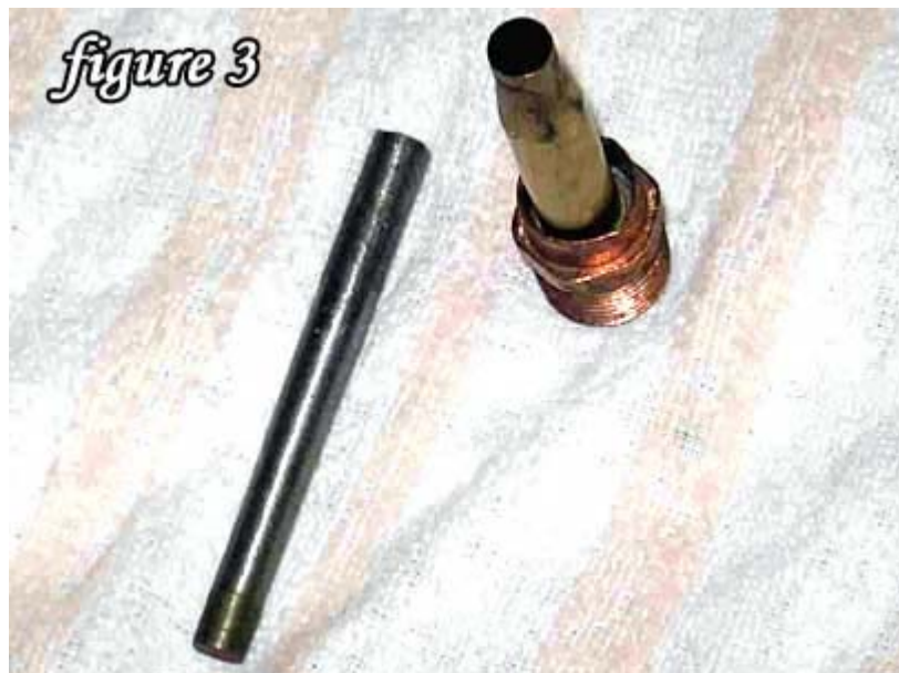
Figure 3. You can use the same base that we used in the 7.5 Swiss article consisting of a 3/8" nut in the coupler.
