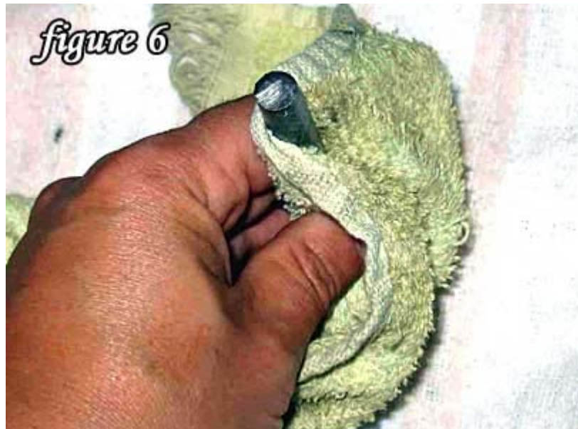
Figure 6. Wrap an old towel around the rod/case mouth to keep the spray from going all over our face. And then smack it with your mallet. You will find that previously reloaded brass will decap quite a bit easier than the original primers.
