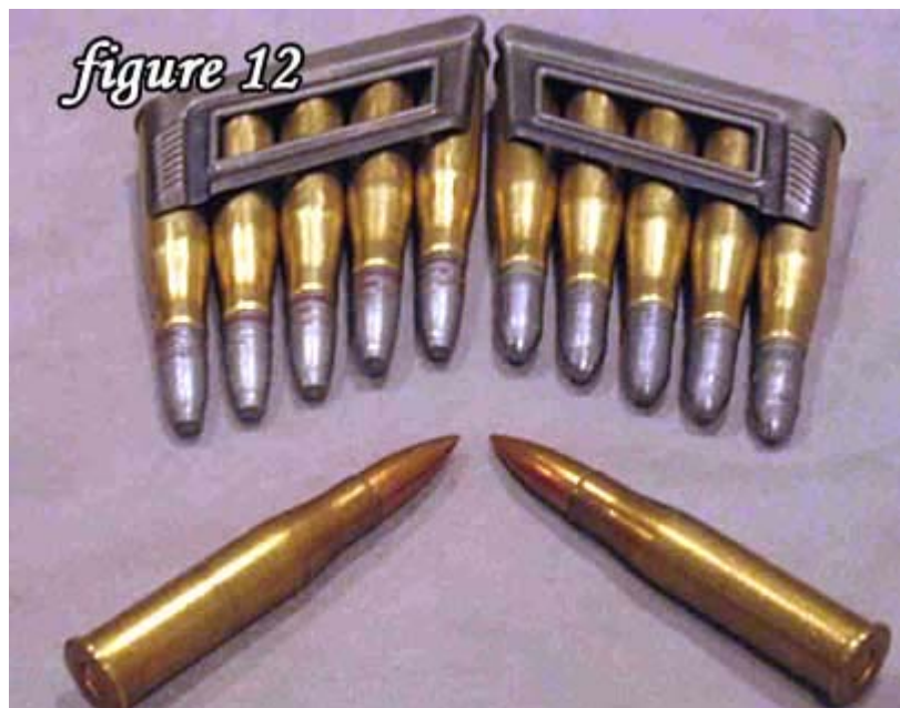
Figure 12. These three types of ammo were used. Center two are mil surp Nazi marked 1938 original ammo. The clip on the left holds Doudna 175gr semi flat nose bullets, the clip on the right holds the Lee # C329-205-1R bullets, cast at about 210gr.
