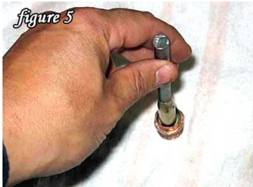
Figure 5. Fill the case with water. Place the case on the base. Insert the rod.
