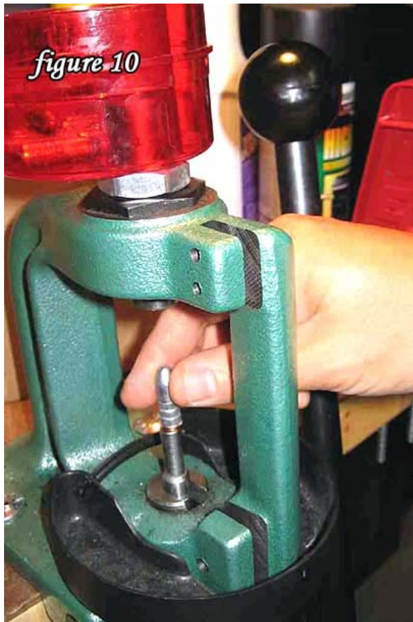
Figure 10. Lee's sizer comes with the sizer die and a base that attaches to your reloading press. You place the lubed/gas checked bullet on the base then run it up into the sizing die. The base of the case serves as a collection bin.
