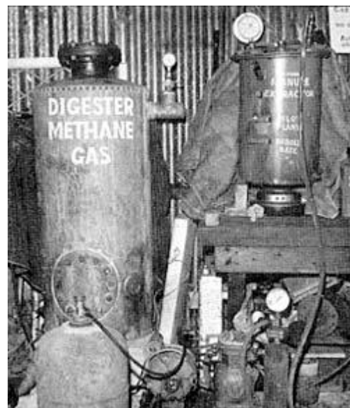
Harold Bate's pilot Manure Extractor and the Manure Digester that he uses for day-to-day generation of automobile and truck fuel. Note the high-pressure compressor with which Bate fills a storage bottle (lower left of photo) to a pressure of 1,100 pounds per square inch.
