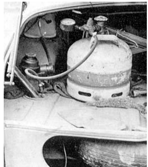
We find secured by another twist of wire the pressure tank of methane which fuels the Bate Hillman. In this case, the tank is a recycled "camping gas" bottle of a type common in England.
