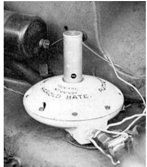
The Bate Auto Gas Converter (demand regulator) as mounted in Harold's 1953 Hillman. The white cover here is purely decoration. Note, again, the rather casual manner in which Bate has installed his accessories in his own car.
