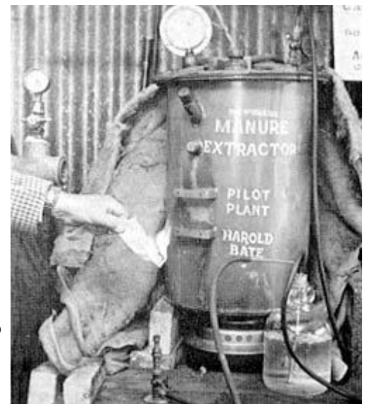
Graphic proof that Harold's small pilot Manure Extractor does the job! Methane from the digester first bubbles into a gallon bottle of water and then passes to a small gas jet where it is easily ignited and supports a flame. Obviously, part of the methane generated by a large digester can be piped to a burner under the extractor for use in maintaining the tank at the optimum gas generating temperature.
