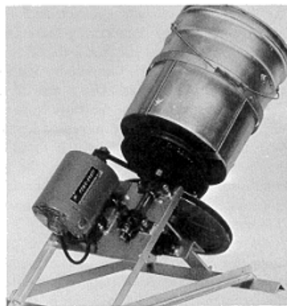
The mixing bucket is equipped with stationary blades that are bent by hand and bolted or riveted inside
