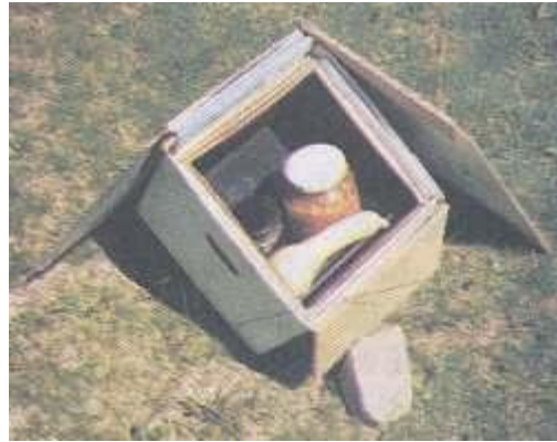
With the collectors back and the glass removed, it's easy to get at the cooked food.
