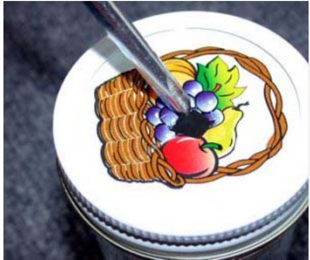
I punched a hole in the soft tin lid, then widened it a bit by moving the screwdriver to the edge of the hole and hitting it again.
