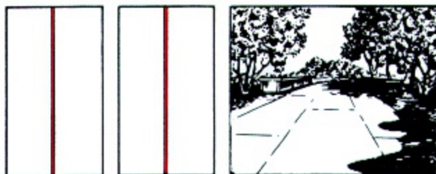
Figure 103. Hard-Surface, Heavy-Duty Road. LARGE-SCALE: Two or three lanes wide. Unless otherwise labeled, the road is two lanes wide. MEDIUM-SCALE: Two lanes wide.
