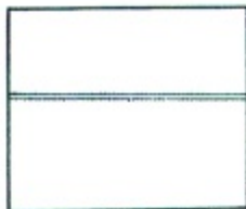
Figure 312. Large Levee and Large Earth Dams. These features are symbolized when they are landmark in nature and an impediment to cross-country movement.
