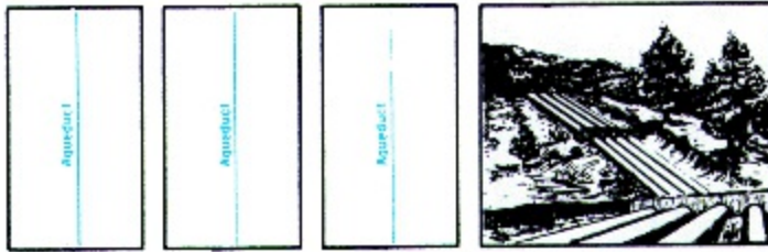
Figure 23. Aqueduct. The symbol represents a conduit used for carrying water. It may be either an open or closed canal. Water pipelines are symbolized by the aqueduct symbol.
