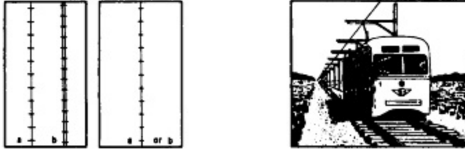
Figure 143. Carline. Carlines are shown only in open areas; they are omitted in built-up areas, streets, and roads. If the line is not in operation, labeling indicates whether it is abandoned, destroyed, or under construction. Single and double-track lines are shown by the same symbol on medium-scale maps. Carlines which are not in operation are symbolized the same as those in operation, except that appropriate labeling is added. Dismantled carlines are shown in the same manner as dismantled railroads. (a) Single. (b) Double.
