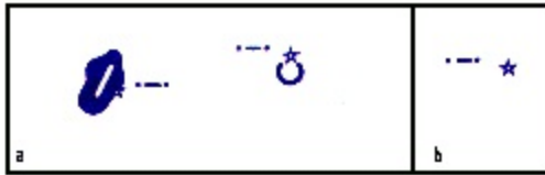
Figure 287. Aeronautical Rotating Light With Flashing Code Identification Light. Symbol is shown as: (a) If located on aerodrome; (b) If in isolated location.
