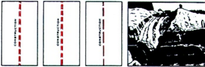
Figure 122. Road Under Construction. Only roads on which construction is actually under way are shown. If information is available, the classification of the completed road is shown by the proper road fill. Proposed roads are omitted.
