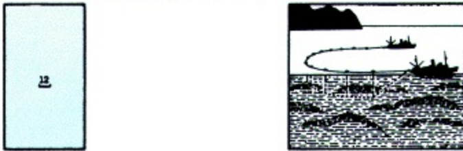
Figure 93. Swept Depth. The figure in the bracket indicates the depth of clearance. This is not necessarily the actual depth. Labeling describes the nature of any danger.
