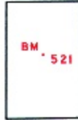
Figure 327. Bench Mark. The symbol represents a described vertical control point established by survey methods of third or higher order accuracy.
