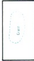
Figure 259. Outlined Landmark Areas. This symbol is used to show areas which are so different in nature or appearance from the surrounding terrain that they serve as outstanding landmarks. The nature of the area is explained by labeling.
