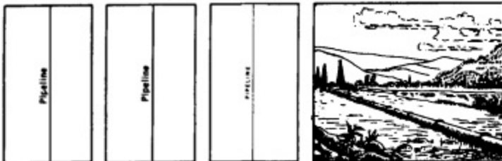
Figure 210. Pipeline. This includes only those pipelines not used for water which are landmark features in areas of sparse culture. They are omitted in developed areas. No effort is made to show pipelines as a continuous feature and only landmark parts are shown.
