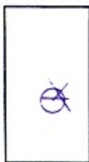
Figure 267. Aerodrome; Runway Pattern Known, Field Limits Unknown. Length of runways shown to scale.
