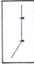
Figure 260. Powerline With Pylons. Pylon symbols are shown at points of directional change, and on straight portions as often as necessary to emphasize the hazard to air navigation.
