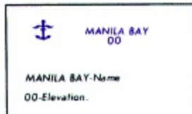
Figure 270. Seaplane-Emergency. This symbol is used to show emergency seaplane landing sites which have no facilities or for which complete information is not available.
