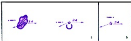
Figure 288. Aeronautical Rotating Light With Course Light and Site Number. Symbol is shown as: (a) If located on aerodrome; (b) If in isolated location.
