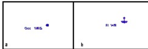
Figure 291. Marine Light With Characteristics of Light. The abbreviations used to show the characteristics are: F (Fixed), Fl (Flashing), QK (Quick Flashing), I QK Fl (Interrupted Quick Flashing), Occ (Occulating), Alt (Alternating), Gp (Group), R (Red), W (White), G (Green), B (Blue), U (Unwatched), SEC (Sector), and Sec (Second). Marine lights are white and alternating lights are red and white unless otherwise labeled. Symbol is shown as: (a) Land light; (b) Lightship.
