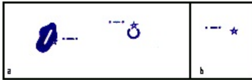
Figure 287. Aeronautical Rotating Light With Flashing Code Identification Light. Symbol is shown as: (a) If located on aerodrome; (b) If in isolated location.
