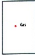
Figure 325. Tank. All types of small tanks which are not shown by the pictotone process are shown by this symbol and labeled as to contents.
