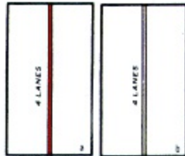
Figure 245. Hard Surface, All-Weather Road, Two or More Lanes Wide. (a) Principal route. (b) Secondary route.
