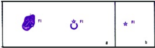
Figure 289. Aeronautical Flashing Light. Symbol is shown as: (a) Located on aerodrome; (b) In isolated location.
