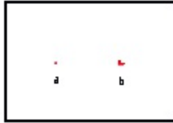
Figure 315. Buildings (1:25,000 and 1:50,000 Scales). Buildings outside the built-up areas which are not shown by the pictotone process are shown as: (a) Small buildings; (b) Larger buildings shown to scale.
