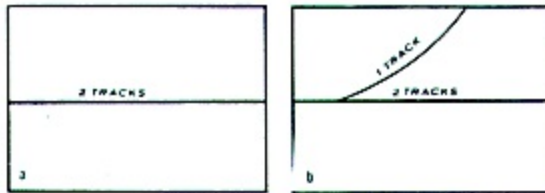
Figure 305. Railroad. All railroads are shown by this symbol with number of tracks indicated by labeling: (a) Railroad; (b) Railroad spur.
