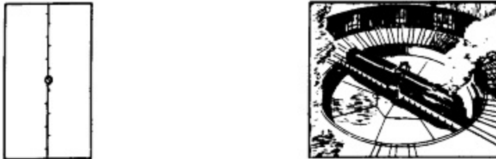
Figure 140. Turntable. A turntable is not drawn to scale. It is usually omitted in congested areas.
