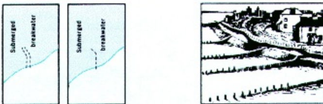
Figure 195. Submerged Breakwater. Breakwaters which are submerged at mean high tide even though exposed at low tide are included.
