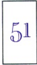
Figure 243. Highest Known Terrain Elevations. The highest known terrain elevations are shown within each 15-minute square as an aid to air navigation. The larger digit represents thousands of feet; the smaller digit represents hundreds of feet.
