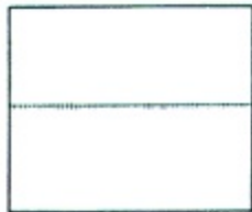
Figure 311. Small Levee. Small levees are symbolized when they are landmark in nature and an impediment to cross-country movement.
