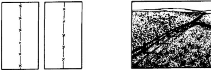
Figure 220. Prominent Fence. Only fences which provide definite landmarks in areas of sparse culture are shown.
