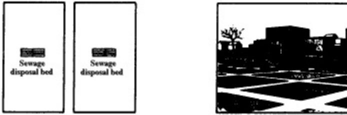
Figure 208. Sewage Disposal or Filtration Bed. These are shown only when they can be plotted to scale. Wherever possible, major separations within the feature are shown. Labeling identifies the feature.
