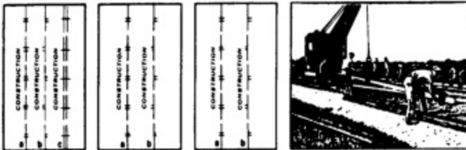
Figure 134. Double- or Multiple-Track Railroad, Nonoperating. Labeling indicates whether railroad is abandoned, destroyed, or under construction. (a) Normal or broad gage. (b) Narrow gage. (c) Standard gage (for use in United States only). Broad gage railroads are labeled as to gage.
