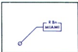
Figure 275. Radio Beacon (R Bn). May also be labeled NDB for nondirectional radio beacons.
