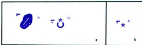
Figure 290. Aeronautical Light With Flashing Code Identification. Symbol is shown as: (a) Located on aerodrome; (b) In isolated location.
