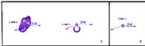
Figure 288. Aeronautical Rotating Light With Course Light and Site Number. Symbol is shown as: (a) If located on aerodrome; (b) If in isolated location.
