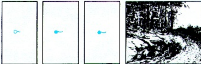
Figure 38. Spring. Springs are shown only in arid areas or where they are important landmark features. When the feature is intermittent, mineral, alkaline, undrinkable, or hot, it will be so labeled.
