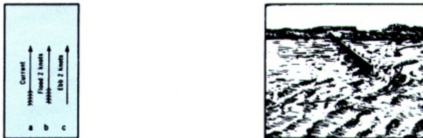
Figure 97. Current. If the speed is known, it is indicated in knots. (a) General. (b) Flood. (c) Ebb.
