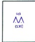
Figure 294. Group Obstruction. Two or more obstructions in close proximity are shown by this symbol. The elevation and height of the highest feature in the group is shown.
