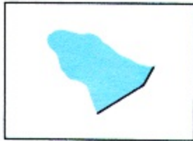
Figure 313. Small Dam. This symbol is used to show small dams of either earthen or masonry construction.
