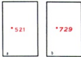
Figure 328. Spot Elevation. (a) Checked elevation established by closed lines, including spirit level, stadia, and vertical angle methods. (b) Unchecked elevation determined by unchecked field surveys.
