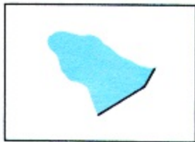
Figure 313. Small Dam. This symbol is used to show small dams of either earthen or masonry construction.
