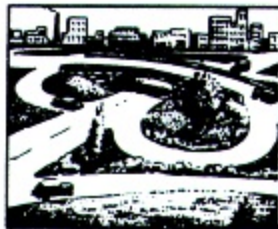
Figure 128. Traffic Circle, Cloverleaf, and Interchange. A cloverleaf is shown to true shape whenever the scale permits. They are sometimes omitted on 1:50,000 scale maps, especially in congested areas. On medium-scale maps the access points on limited-access roads are the only cloverleaves shown.
