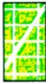
Figure 301. Street (1:25,000 and 1:50,000 Scales). Streets are shown by a solid white line .02'' wide, or if wider, drawn to scale.
