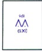
Figure 294. Group Obstruction. Two or more obstructions in close proximity are shown by this symbol. The elevation and height of the highest feature in the group is shown.
