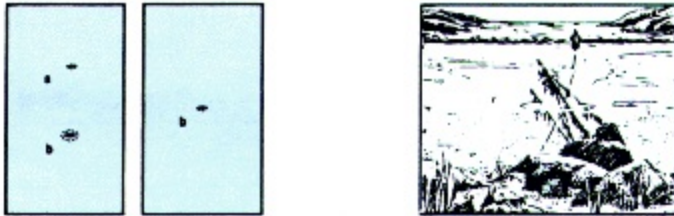
Figure 88. Sunken Wreck. The symbol represents wrecks which are less than 10 fathoms (60 feet) deep, with no part of the hull above water at the hydrographic datum. Masts may or may not be above water. The center of the symbol marks the location of the wreck. Only actual dangers are shown on medium-scale maps.
