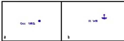
Figure 291. Marine Light With Characteristics of Light. The abbreviations used to show the characteristics are: F (Fixed), Fl (Flashing), QK (Quick Flashing), I QK Fl (Interrupted Quick Flashing), Occ (Occulating), Alt (Alternating), Gp (Group), R (Red), W (White), G (Green), B (Blue), U (Unwatched), SEC (Sector), and Sec (Second). Marine lights are white and alternating lights are red and white unless otherwise labeled. Symbol is shown as: (a) Land light; (b) Lightship.
