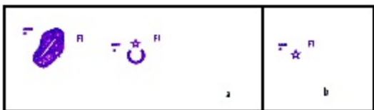
Figure 290. Aeronautical Light With Flashing Code Identification. Symbol is shown as: (a) Located on aerodrome; (b) In isolated location.
