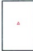
Figure 326. Triangulation Station. The symbol represents a described horizontal control point which is marked on the ground and which was established by triangulation or traverse of third or higher order accuracy.
